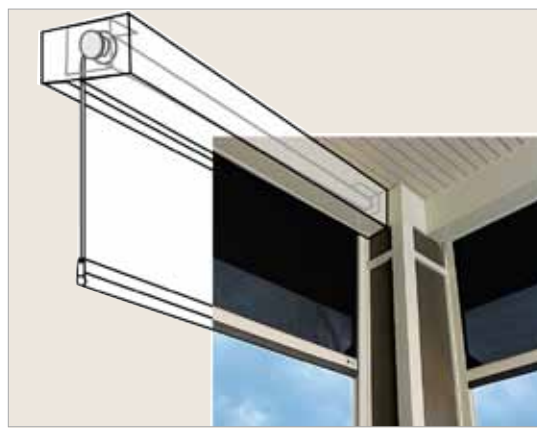
Recessed mount with detail of contents of cavity.
