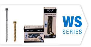
The **WS Wood Screw** is a self-drilling screw used for numerous framing applications. This screw features a reverse locking serration on the bottom of the screw head to help prevent over tightening against a steel plate. The USP head stamp identifies screws for easy inspection.
